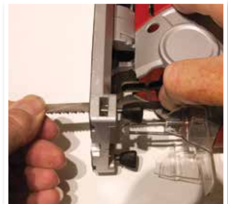
Walter Hall fitting the CMT blade to the jigsaw
