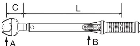
A number of variables will affect the accuracy of the above calculation: length of the adapter or extension, length of the wrench and variations in hand position.
