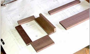
This is what I am working on. The "L" on the right is made up of the two stiles I just profiled with the locking miter bit.
