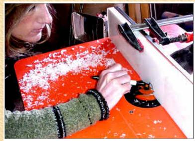
While we had used the other two cutters before, we had not used the raised panel cutter with the new Sommerfeld fence. Beth is marking a new insert with the profile of this bit.
