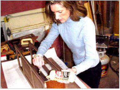
Beth uses a brush to spread the carpenter's glue thoroughly over the tongue. There is a lot of gluing surface in this joint. It makes sense to use it. With the glue spread, she adds the side and turns the assembly over to glue the other side.
