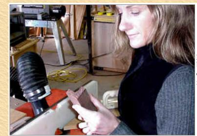
Beth inspects her corner pieces. They fit together perfectly and give a sharp, square outside corner. What's best is that the sides are already the 1/2'' stock, so they can now be routed with the rail and stile cutters to fit the rest of the frame section.
