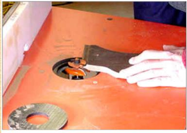
With each of the panels at their right dimensions and shapes, I am ready to cut the raised panel profile. I start by installing the junior raised panel bit. Here I am adjusting the bit height using the tongue of the coped end to help me "eyeball" the height. I have lowered the router speed. This is a 2 1/2" bit and the maximum speed for that diameter is 16,000.
