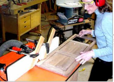
Having made the sample cut and positioning a couple of featherboards to keep the panel flat on the table, Beth makes the tongue cut on the edge of both the front and back panels.
