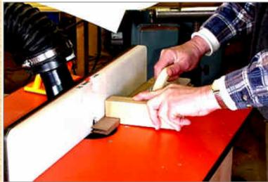
Here I am running the stock. My left hand keeps pressure on the piece so that it is on the table and against the fence. My right hand is using the MDF pushblock to push the piece through the cutter.
