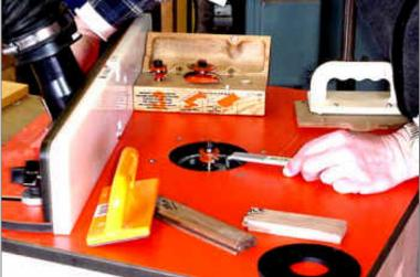
I tighten the bit using the bent wrench.
