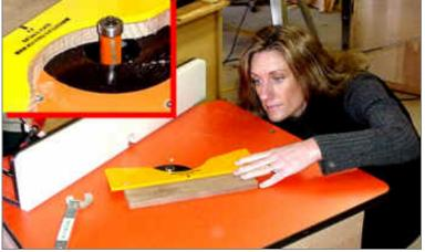
She has installed a trim bit so that the bearing is in contact with the template and the cutter covers the wood. The inset shows a closer, "birdseye" view. Beth makes her cut. When she is coming up against the cross grain, she is careful to take minimal cuts and little pressure letting the cutter do its work. A very sharp cutter and not pushing it greatly reduces the chip out problem.
