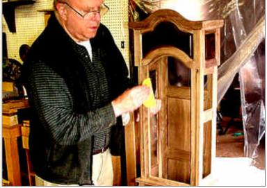
This is a good time to sand of few of the edges that haven't yet been touched. I am "feathering" the edges of the door recess. A couple of days later and Beth is back. We are trying to figure out the instructions for mounting the clock mechanism. The clock dial will go behind this frame and be attached to it.
