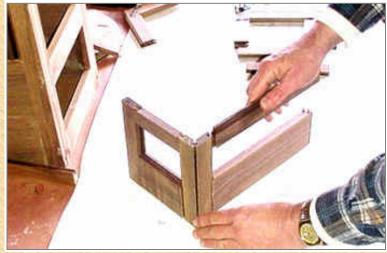
I am only dry fitting at this point and want to give you an idea of how the sections go together. The locking miter joint, we did first, will be the corner post. [Note, the gap at the corner is because I am not holding the corner together.]
