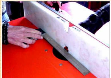
Lastly, she adjusts the fence using the straight edge to align the fence with the pattern bearing.
