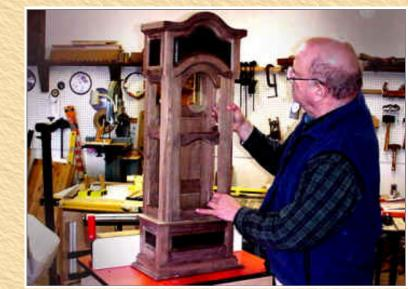
I am holding the door in place. I have to find overlap hinges that will look right in this piece. Next, I have to mount the stage for the clock itself. Then we can move to the warmth (yea!) of the house for the finishing steps.
