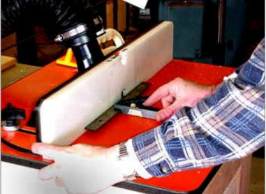
With the router turned off and the bit at a complete stop, I align the fence with the top bearing and lock it in place.
