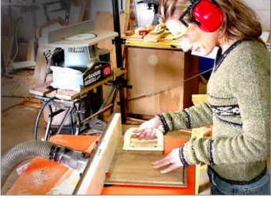
With the fence insert cut, she starts the cutting of the panels by making shallow cuts and then moving the fence back until the bearing is aligned with the fence. She cuts the end grains and then the long sides. This minimizes tearout.
