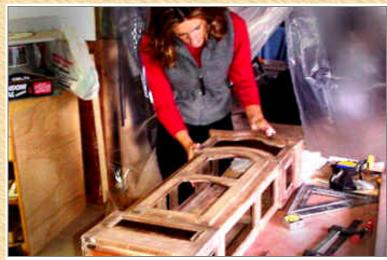
Now she can slide the top assembly over the top of the case. The door is not mounted yet but is in place to help Beth locate the top exactly.
