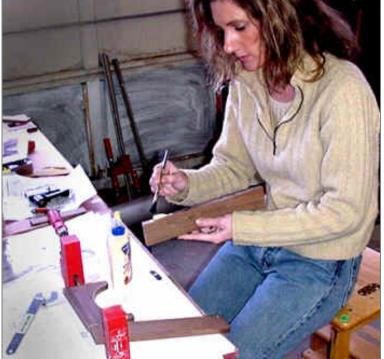
Beth has become expert at gluing and clamping these frame assemblies together.
