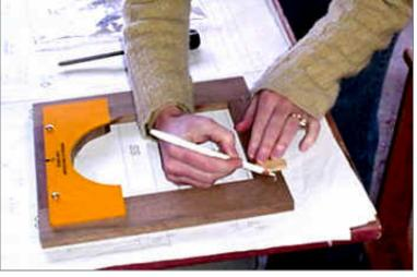
The bottom rail is too narrow for any of the biscuits we have, so Beth has cut down a #20 biscuit. The bottom of the rail will be out of sight, so she makes her mark favoring that side. With the 5/32" slot cutter mounted in the router, Beth eases the pieces into the cutter at the marks.
