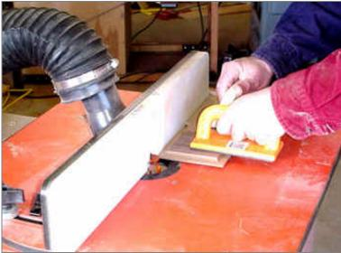
Using the two push block method that I have used in the earlier procedures, I cut the raised panel profile on each of the square panels.
