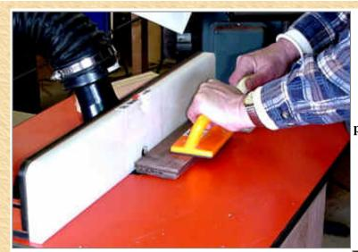
For the wider rails, I switch back to the standard pushblock.
