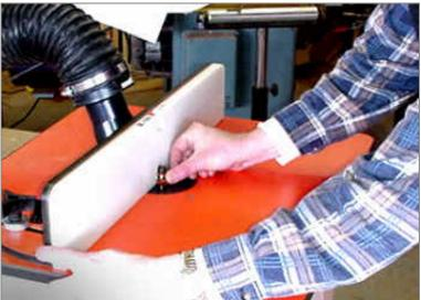
I move the fence forward to see that the bit does, in fact, clear the opening as I manually rotate the bit.
