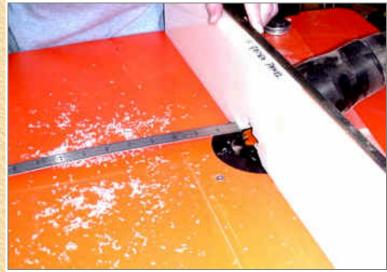
Beth adjusts the fence so that the cutter depth is 1/4". She has raised the router so that the cutter is 1/8" above the table.
