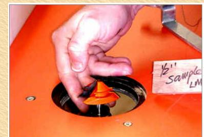
I have installed the locking miter bit. I have also brought out my sample that I cut from the same stock. I will use that to setup the router bit height and fence depth.
