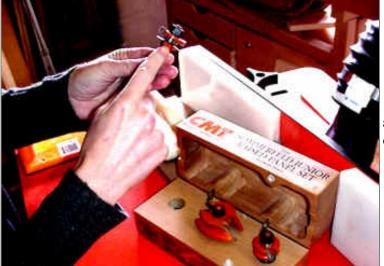
It is time to cut the cope ends on all the rails of the sides and the front panel. She selects the cope cutter it is the one with the bearing in the middle.
