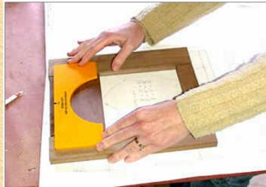
The plans say to glue up the frame and then use the template for shaping the upper rail. While that will give us a larger piece to hold when routing, we decided that we should make the rough cut at the bandsaw before we glue the pieces together. Of course we could use a saber saw to make the rough cut after the glueup.
