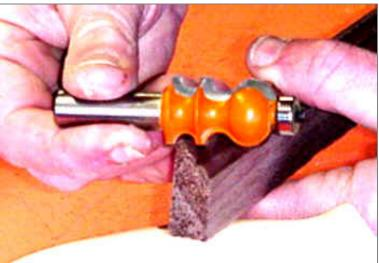
I make the second, rounding over pass using just this one section of the multi-profile bits. I have several of those and it always amazes me when I can make use of just a bit of it. It saves the day this time.
