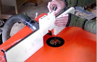
She installs the fence insert that has been cut for this bit.
