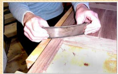
The cabinet scraper quickly removes the little trace of glue squeeze out.
