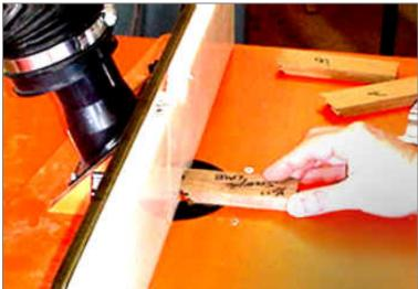
When the router comes to a complete stop, I move the fence into the bit and use the sample cut to adjust the fence depth.
