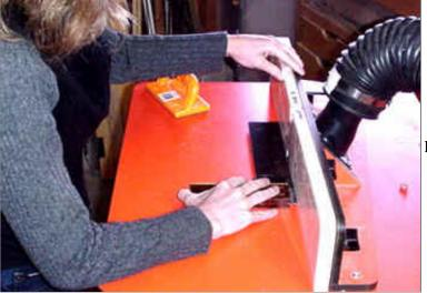
She brings the fence forward until it is aligned with the pattern bearing and locks it in place.
