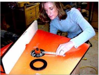
With the grooves cut in the sides, Beth now installs the other cutter. This one will be adjusted so that it cuts a tongue that is centered on the 1/2'' frame stock.
