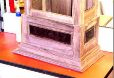
The two pieces of base molding are installed and look just fine. Now to attack the molding for just above the bottom raised panel frame. This is the one we were having trouble with yesterday. This is what I am going to do. I have already cut a "classic ogee" profile. It leaves a sharp, square edge. I have marked the bull nose edge that I think I want.
