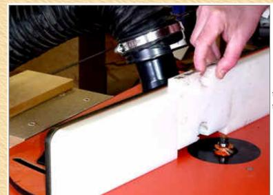
The correct fence insert is installed. Since I have cut this insert in the other edge of the same insert, all I have to do is switch it end for end.
