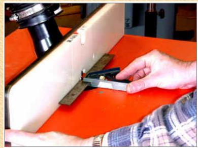
I now use a straight edge to align the fence with the pattern bearing. I lock the fence in place and, one more time, rotate the bit to be sure that it is free to move. With that done, I am ready to cut the cope ends on the rails.
