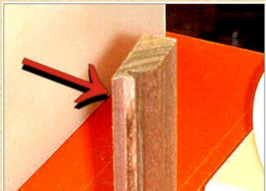
This is the cut. The arrow points to the outside edge which should be knife sharp. If there is any width to it, the fence needs to be backed off slightly.
