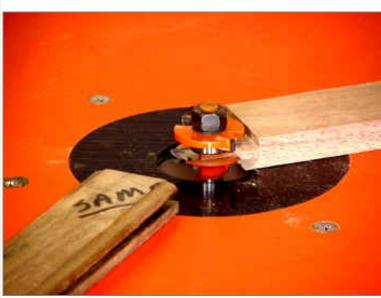
I have installed a throat plate and am now setting the router bit height using the coped end of my sample. Now, I install the fence insert with the shape cut-out for that bit. Having marked the top helps to identify the correct insert.
