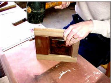
She carefully taps the stile back onto the assembly. She then flips it around and removes the other stile, glues and reassembles. Not only does this keep all the parts in order, but it is much easier to manage. She places the side panel in the clamps to dry. Note that she has a front panel clamped as well. This is not glued at this point. It is in the clamp to mate with the locking miter corner to keep the corner from being crushed by the clamp.
