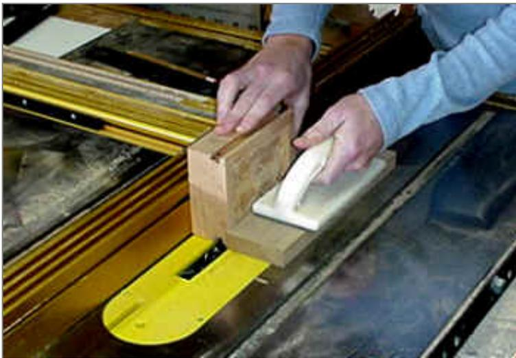
Deciding that the two sides should be at an angle of  $15^\circ$ , Beth has installed the stacked dado set and set the blade tilt angle to  $15^\circ$ . She uses a push shoe to guide the box over the dado set.
