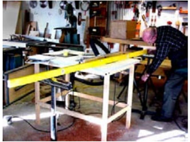
Here I am edging an eight footer of curly maple. With the left hand keeping the board against the fence and the right hand feeding the board, the jointing goes smoothly.
