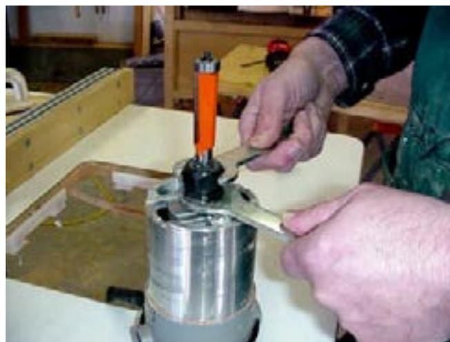
Then, install the router and adjust the fence so that the left-side of fence is in exact alignment with the straight bit bearing. The gap between the straight edge and the right fence should equal the Formica shim thickness. Be sure to move the two fences as close as possible to the bit—as a matter of practice, I leave about 1/8" space around the bit.
