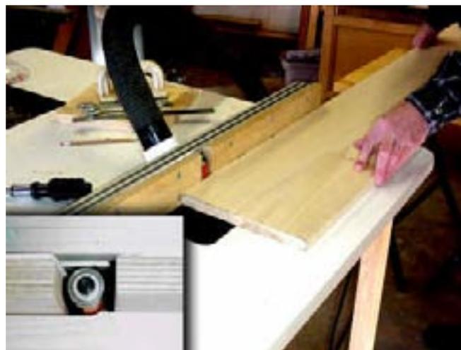
When I am joining boards, I first place them together and mark the boards with a light "arc" witness mark. Then, I run one board with the mark down and the other one with the mark facing up. This way, if the router is not exactly 90 degrees, the joint will still be perfect. I do this when using the jointer as well.
