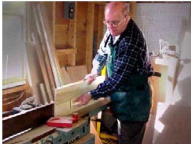
If your router table has a split fence as does this one from Woodhaven, it is a simple matter of loosening the screws on the left hand side and slipping in shim material. I use a scrap of Formica in which I have cut slots to go around the screws. There are many ways to shim the left hand fence out. For me, using Formica is fast, simple and accurate. I just slide the shim in place and re-tighten the screws.
