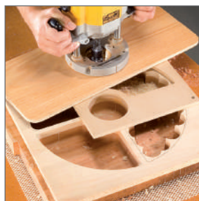
Rout the interior to final shape using the bowl and tray router bit and collet extension.
