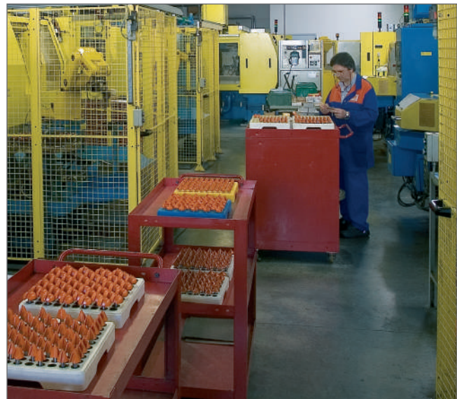
Loading the automated multi-axis CNC sharpening machines.
